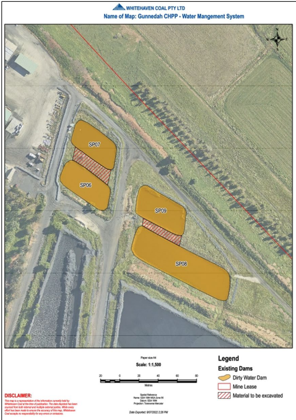
Figure 5 Settling Pond Augmentation
